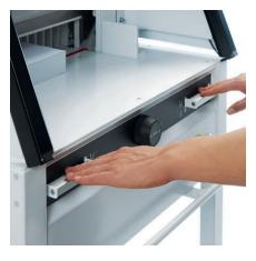
PATENTED EASY-CUT ACTIVATING BARS Blade and clamp can be activated independently via the two-step blade activating bars with separate trigger points for blade and clamp.
