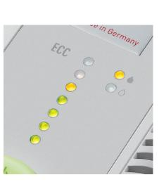
**ECC - ELECTRONIC CAPACITY CONTROL** This electronic feature indicates the used sheet capacity during shredding process to avoid paper jams.
